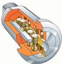
In addition to designing a lock that provides a high level of security, ASSA Desmo realizes the need for ease of function. The Precision Drive Pin System operates completely independent of springs. The pins are 100% guided by the operation of the key ensuring accurate, secure, and long lasting performance. The face of the lock and the tip of the key are shaped to guide key entry. This feature increases the ease of use, especially in hard to reach lock applications.
